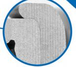
No gap on the roll form of WJB's hub assemblies, which outperformed value grade aftermarket roll formed hub assemblies with visible gap.
